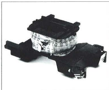
Fig. 2. Contactor coil with burnt out winding
